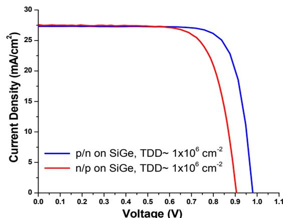
Figure 1: Illuminated AM0 I-V response for p<sup>+</sup>n and n<sup>+</sup>p GaAs cells grown on v-Ge substrates with close TDD values. Note the difference in Voc. The p<sup>+</sup>n AM0 efficiency is 15.6% and the n<sup>+</sup>p cell is 13% efficient. AM1.5 values will be ~ 2-3 absolute percent higher.
