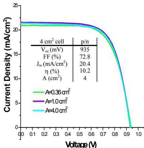
Figure 3. AM0 I-V data for GaAs/v-Ge cells with areas of 0.36 cm<sup>2</sup>, 1 cm<sup>2</sup> and 4 cm<sup>2</sup>. Inset shows total area cell data for the 4 cm<sup>2</sup> cell (7% grid coverage). No AR coatings have been applied.
