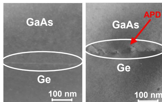
Figure 2. Cross sectional TEM images of GaAs/Ge epilayer interfaces, with (left) and without (right) an MEE GaAs nucleation step.
